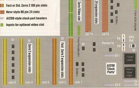
The dozen expansion ports and sundry are distributed around the Z4 backplane, with several empty sockets to allow the interface logic to be implemented with different chips if component supplies are typically erratic.
