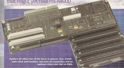
he problem with an A1200 is its limited expansion potential. Apollo aim to cure this, with an expansion backplane boasting a dozen expansion slots - five largely compatible with the 16-bit Zorro II standard, two new 32-bit Z4 sockets, four eight bit ones, based on the much-perverted A1200 internal 'clock port', and an optional
